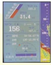
The NAV data screen shows own ship's position, speed, distance run, waypoint data with wpt number, range/bearing to wpt and XTE, water depth and temperature.
